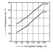
2. Ambient temperature characteristics Sample: JM1aN-TMP-DC24V, 5 pcs.
