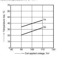
2-(3). Coil temperature rise (4 Form C/AC type) Measured portion: Inside the coil Ambient temperature: 70°C 158°F
