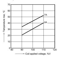
2-(2). Coil temperature rise (2 Form C/DC type) Measured portion: Inside the coil Ambient temperature: 70°C 158°F
