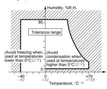
(3) Atmospheric pressure: 86 to 106 kPa Temperature and humidity range for usage, transport, and storage:2) Condensation
