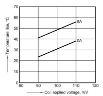
2-(4). Coil temperature rise (4 Form C/DC type) Measured portion: Inside the coil Ambient temperature: 70°C 158°F
