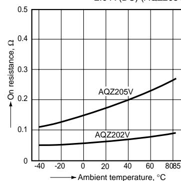
**3.-(2) On resistance vs. ambient temperature characteristics**
