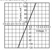
9. Off state leakage current
