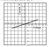
9. Off state leakage current
