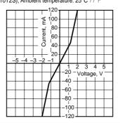
9. Off state leakage current
