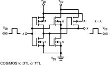
Hex COS/MOS to DTL or TTL converter (inverting). Connect  $V_{CC}$  to DTL or TTL supply. Connect  $V_{DD}$  to COS/MOS supply.
